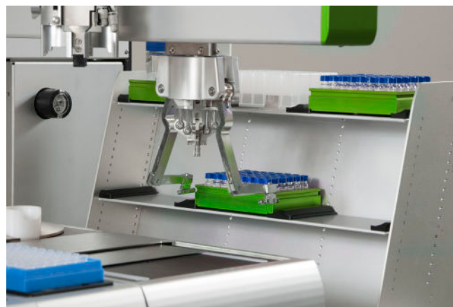
Figure 2: Junior for powder dispense taking a plate from the integrated shoulder hotel to the balance.
