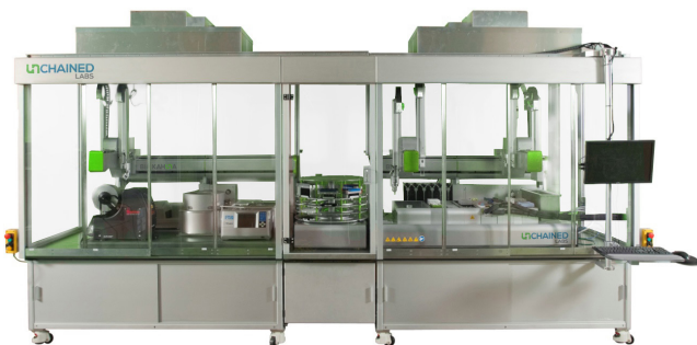
Figure 1: The Big Kahuna system configured for biologics formulation. The robot on the right prepares formulations and measures pH, viscosity and visual inspection. The left robot integrates with the Wyatt DynaPro II dynamic light scattering (DLS) instrument and Molecular Devices SpectraMax microplate reader. A low-bioburden HEPA enclosure encapsulates the system.
