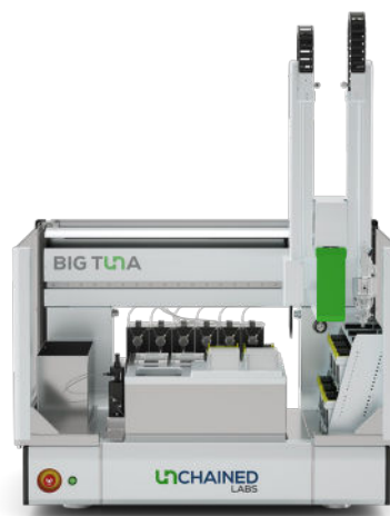
Figure 1: Big Tuna automates buffer exchange.
