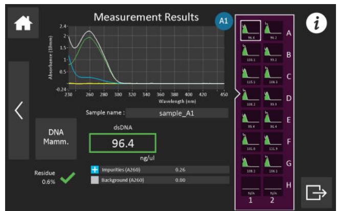
Figure 4: Illustration of the Results screen on the Little Lunatic. Unmix app results of the selected sample are shown as spectral shape as well as in calculated values. Additional impurity and/or background detailing will be reported if possible.
