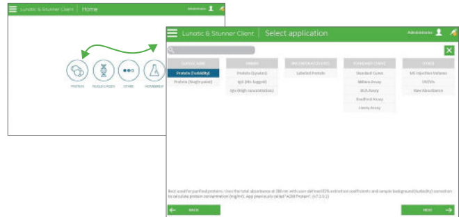
Figure 1: Illustration of the Lunatic interface. The image in the back shows the Sample Type screen whereas the image in the front displays the available applications for the selected Sample Type.
