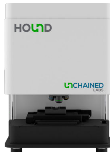
Figure 1: Hound counts and identifies the composition of visible and sub-visible particles with both automated and manual modes. Hound uses Raman (532 nm and 785 nm) and LIBS to identify the composition of particles, helping users track down the particle source.
