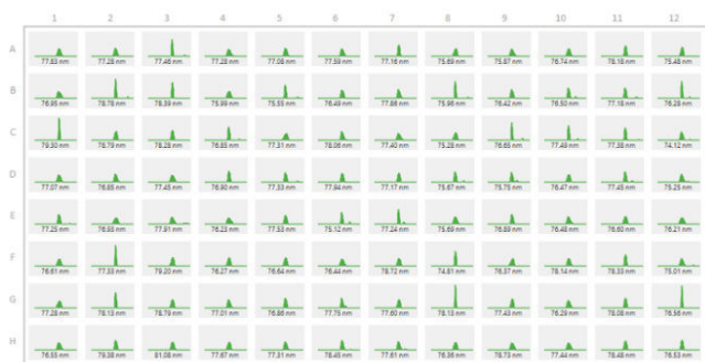
Figure 4: Stunner's DLS determines the size and size distribution on 96 samples of LNPs in about 1 hour.
