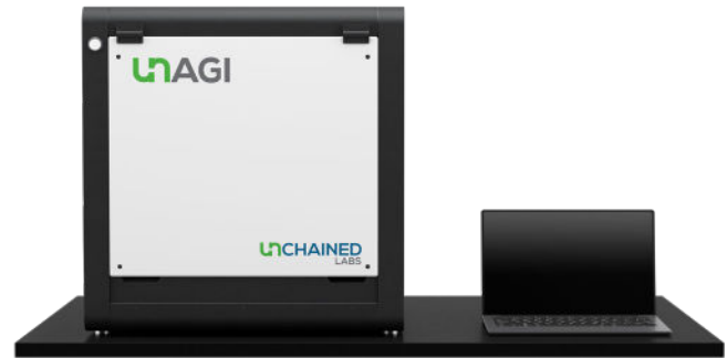
Figure 1: Unagi is your automated benchtop buffer exchange and concentration solution for up to 8 unique samples between 0.5 – 48 mL.
