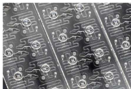
Figure 1: Lunatic is the next-generation UV/Vis system for nucleic acid (and protein) quantification (A). High Lunatic plates have 96 individual microfluidic circuits that only use 2 \mu L per sample and read up to 96 samples at a time (B).
