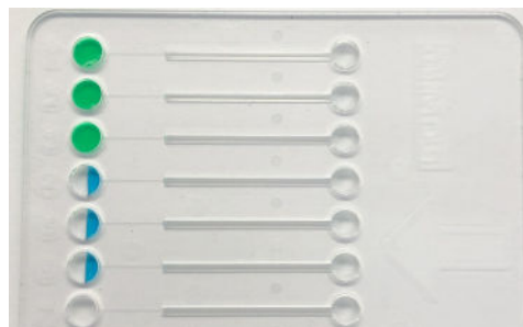
Figure 1: Honeybun (A) is the only rapid microvolume viscometer and rheometer for proteins, vaccines, viral vectors and injectables. Honeybun and its consumable Bun (B) read up to ten samples in minutes with just 35 \mu L (Channels 1–3) or 15 \mu L (Channels 4–6) of sample.
