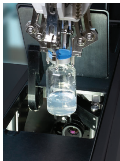
Visual inspection for turbidity, particle, color
